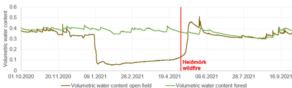
Fig. 5 Volumetric water content in soil in pine forest (green) and open field (brown) from 1.10.2020 to 1.10.2021 measured in the water protection area ML. The vertical line shows the timing of the wildfire.
