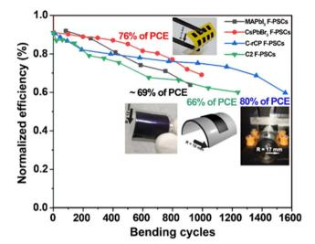
Fig. 6 Bending test of FC-PSCs.
