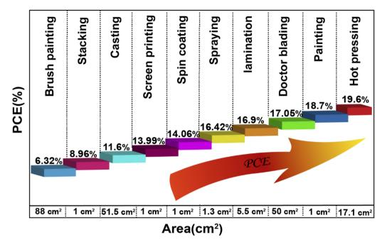
Fig. 4 Top PCEs measured for large-area (≥1 cm²) C-PSCs using various scalable deposition methods for carbon electrodes.<sup>42,80,98–105</sup>
