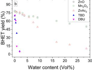
Fig. 1 The influence of water content (vol%) on PET conversion (a) and the yield of BHET(b) when using five different catalysts: ZnO (zinc oxide),  $Mn_2O_3$  (manganese(III) oxide),  $ZnAc_2$  (zinc acetate), TBD (1,5,7-triazabicyclo[4.4.0]dec-5-ene), and DBU (1,8-diazabicyclo[5.4.0] undec-7-ene). (Operating conditions: temperature = 190 °C, reaction time = 2 h, catalyst loading = 1 wt%, EG volume = 25 mL, water content = 0–30 vol%).
