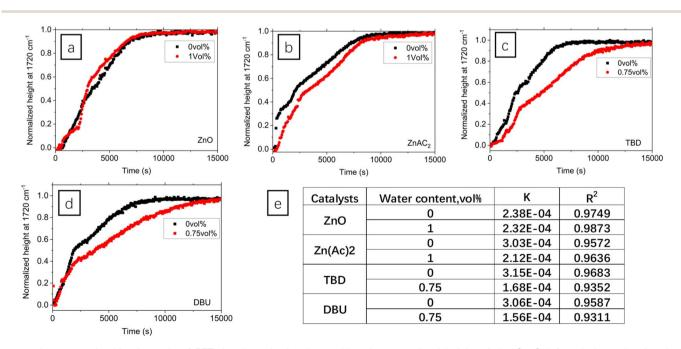
Fig. 4 A comparative kinetic study of PET depolymerization by tracking the normalized height of the C=O infrared absorption band at 1720 cm<sup>-1</sup> (representing BHET concentration) as a function of reaction time for four distinct catalysts: ZnO (a), ZnAc<sub>2</sub> (b), TBD (c), and DBU (d) and the corresponding K value for different conditions (e).
