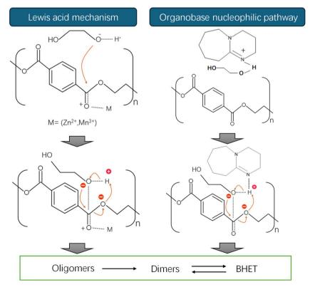
Fig. 6 Comparison of Lewis acid and organobase nucleophilic pathways for PET depolymerization.
