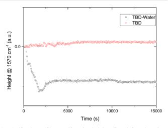
Fig. 5 Kinetic profiles tracking the height of an infrared peak at 1570 cm<sup>-1</sup>, which corresponds to the C=N stretching vibration of the TBD catalyst.
