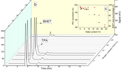
Fig. 2 (a) Chromatogram of products from the ZnO-catalyzed PET depolymerization with 28 vol% water, (b) a series of HPLC chromatograms illustrating the PET depolymerization process catalyzed by ZnO under varying water content conditions (0, 2, 6, 10, 12, and 28 vol%) and (c) the corresponding peak area percentage of BHET among all products and PET conversion. (HPLC conditions: C8 column, UV detector 254 nm, mobile phase = methanol/water (7 : 3 v/v), temperature = 25 °C).
