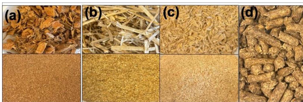
Fig. 1 Representative image of the different feedstocks (a) coconut chips, (b) hay, (c) rice hulls, and (d) 4-crop mix as such (top panel), and when ground to 2 mm size (bottom panel).
