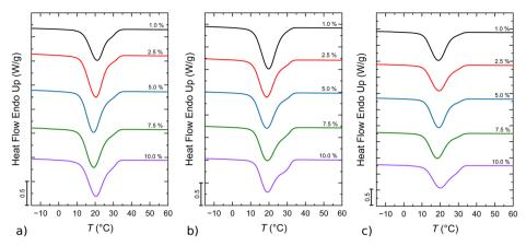
Fig. 1 DSC cooling curves at  $20 \, ^{\circ}\text{C}$  min $^{-1}$  of PCL composites with (a) NdFeB, (b) SFO, and (c) SFO-CFO magnetic micro- and nanoparticles in the composition range of 1-10%.
