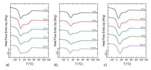
Fig. 2 DSC cooling curves at 20 °C min<sup>-1</sup> of PBSA composites with (a) NdFeB, (b) SFO, and (c) SFO-CFO magnetic micro- and nanoparticles in the composition range of 1–10%.
