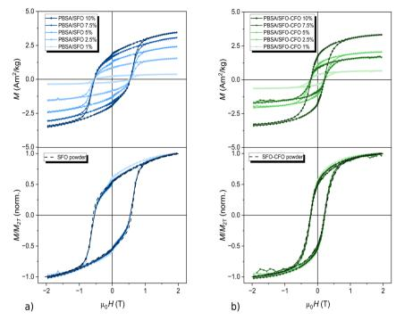
Fig. 9 Field-dependent magnetization loops of (a) SFO and (b) SFO-CFO PBSA-based composites normalized to entire mass (upper panel) and normalized to  $M_{2T}$  (bottom panel). All measurements were performed at 300 K.
