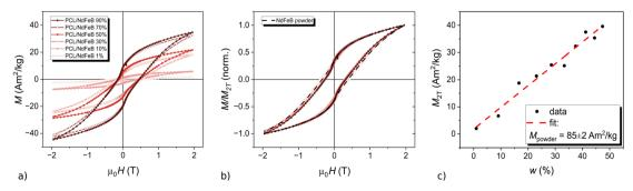
Fig. 8 (a) Field-dependent magnetization loops of PCL/NdFeB composites in the filler loading (C) range of 1–90% measured at 300 K (selected samples are shown); (b) the same curves normalized to magnetization measured at the applied field of  $2 T (M_{2T})$  and horizontally shifted to ease comparation with the pure powder (dashed black line); (c)  $M_{2T}$  as a function of filler mass fraction.
