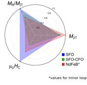
Fig. 7 (a) Field-dependent magnetization loops of M(N)Ps (SFO – blue, SFO-CFO – green, and NdFeB – red); (b) a radar diagram comparing the normalized magnetic properties of the powder samples. Note that a minor loop was recorded for the NdFeB powder. Each property magnetization at 2 T ( $M_{2T}$ ), remanence ratio ( $M_R/M_{2T}$ ), and coercivity ( $\mu_0H_C$ )—was normalized to the maximum value observed for that property across all samples. Measurements were performed at 300 K.
