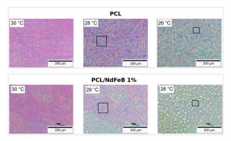
Fig. 4 PLOM micrographs of (upper panel) PCL homopolymer and (bottom panel) PCL/NdFeB composite (C = 1%) at 30 °C, 28 °C, and 26 °C. Black boxes show differences in spherulitic average sizes between neat PCL versus the composite. In neat PCL, within the selected area of each box, the average spherulitic size is slightly larger.
