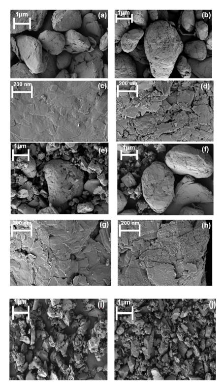
Fig. 7 FESEM of Gr (a) and (c) before and (b) and (d) after heat treatment, Si-Gr@Gr (e) and (g) before and (f) and (h) after heat treatment and Si-Gr (i) before and (j) after heat treatment (magnification of (a), (b), (e), (f), (i) and (j) is  $5k \times$  while (c), (d), (g) and (h) are at a magnification of  $25k \times$ ).
