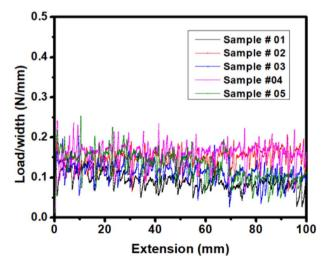
Fig. 10 Peel strength of the Si-Gr@Gr electrode.
