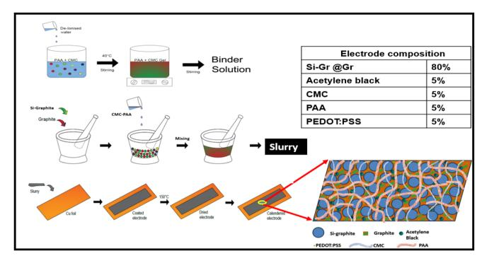
Fig. 1 Preparation of a Si-Gr@Gr anode.
