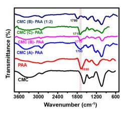
Fig. 2 FTIR spectra of CMC, PAA and CMC-PAA with different grades of CMC and proportions.
