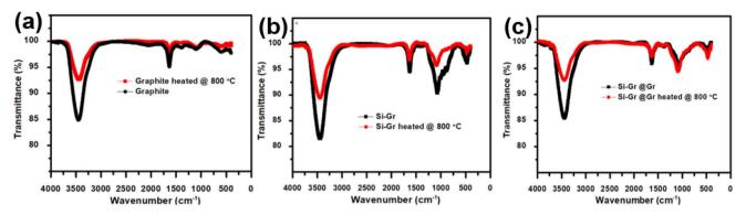
Fig. 4 FTIR spectra of (a) graphite, (b) Si-Gr and (c) Si-Gr@Gr before and after heating at 800 °C.
