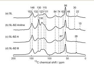
Fig. 6 Solid-state  $^{13}$ C CP MAS NMR spectra of (a) SL, (b) SL-BZ-aniline, (c) SL-BZ-A, and (d) SL-BZ-B. Chemical shift values (in ppm) of each peak are indicated.
