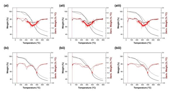
Fig. 15 TGA thermograms collected for (a(i)) SL-BZ-aniline, (a(ii)) SL-BZ-A, (a(iii)) SL-BZ-B, (b(i)) SL-PhBZ-aniline, (b(ii)) SL-PhBZ-A and SL-PhBZ-B (dark red and grey). Thermograms for (a) SL and (b) SL-Ph are shown in light red and black in each graph for comparison.
