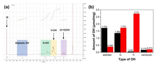
Fig. 8 (a) Liquid-state <sup>31</sup>P NMR spectra recorded of SL-Ph. (b) Graph summarising the amounts of each type of OH group in SL before (black) and after (red) phenolation of SL, according to comparison with the internal standard.
