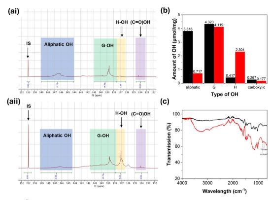
Fig. 10 (a) Liguid-state <sup>31</sup>P NMR collected of phosphitylated (i) KL and (ii) and KL-Ph. (b) Graph summarising the amounts of each different OH group present in KL before (black) and after (red) phenolation. (c) FTIR spectra of KL (black) and KL-Ph (red)
