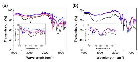
Fig. 12 FTIR spectra of unmodified (a) SL-Ph (black), SL-PhBZ-aniline (purple), SL-PhBZ-A (red) and SL-PhBZ-B (blue) and (b) KL-Ph (black), KL-PhBZ-aniline (purple), KL-PhBZ-A (red) and KL-PhBZ-B (blue).
