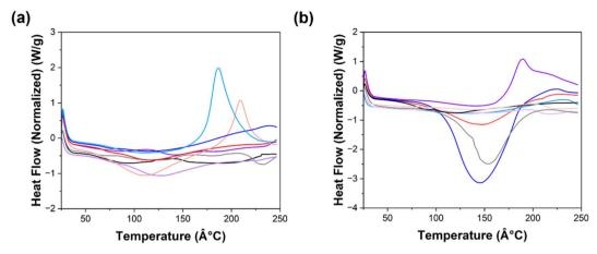
Fig. 17 DSC curves collected for (a) SL (black), SL-Ph (grey), SL-BZ-aniline (purple), SL-PhBZ-aniline (purple), SL-PhBZ-A (red), SL-PhBZ-A (pale red), SL-BZ-B (blue), SL-PhBZ-B (pale blue); (b) KL (black), KL-Ph (grey), KL-BZ-aniline (purple), KL-PhBZ-aniline (pale purple), KL-BZ-A (red), KL-PhBZ-A (pale red), KL-BZ-B (blue), KL-PhBZ-B (pale blue).
