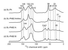
Fig. 13 Solid-state <sup>13</sup>C CP MAS NMR spectra of (a) SL-Ph, (b) SL-PhBZ-aniline, (c) SL-PhBZ-A, and (d) SL-PhBZ-B. Chemical shift values (in ppm) of each peak are indicated.
