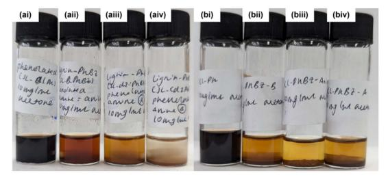
Fig. 14 Photographs of (a(i)) SL-Ph, (a(ii)) SL-PhBZ-aniline, (a(iii)) SL-PhBZ-A, (a(iv)) SL-PhBZ-B, (b(i)) KL-Ph, (b(ii)) KL-PhBZ-aniline, (b(iii)) KL-PhBZ-B, (b(ii)) KL-PhBZ-B, (b(iii)) KL-PhBZ-B, (b(iii)) KL-PhBZ-B, (b(iii)) KL-PhBZ-B, (b(iii)) KL-PhBZ-B, ( PhBZ-A and (b(iv)) KL-PhBZ-B dissolved in acetone (10 mg mL<sup>-1</sup>) by stirring at room temperature for 10 minutes before leaving any undissolved solid to settle.
