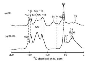
Fig. 11 Solid-state <sup>13</sup>C CP MAS NMR spectra of (a) Sonichem lignin and (b) phenolated Sonichem lignin. Chemical shift values (in ppm) of each peak are indicated.
