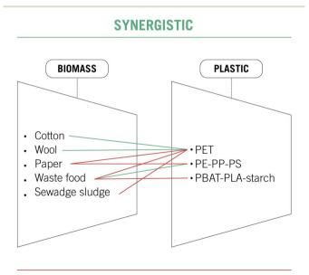
Fig. 4 Synergistic and non-synergistic effects of mixing plastic and biomass in waste processing technologies. PET: polyethylene terephthalate; PE: polyethylene; PP, polypropylene; PS: polystyrene; PBAT: polybutylene adipate terephthalate, PLA: polylactic acid.
