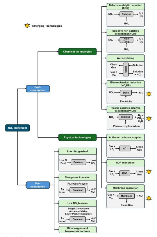
Fig. 3 Simplified schematics for current and emerging NO<sub>x</sub> abatement technologies.
