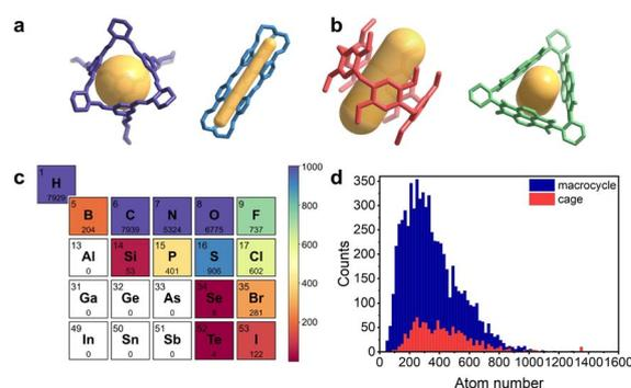
Fig. 2 (a) Examples of cages in MCD. (b) Examples of macrocycles in MCD. The voids within cages and macrocycles are highlighted in yellow. (c) The number of macrocycles and cages in the MCD containing specific elements. (d) Distribution of atomic numbers per unit cell across the structures in the MCD.
