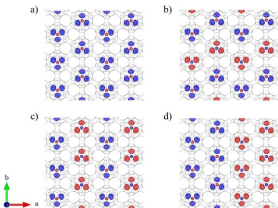
Fig. 2 Spin density of considered magnetic configurations for  $V_3N@C_{80}$ . (a) Ferromagnetic (FM), (b) zig-zag, (c) single-stripe and (d) double-stripe antiferromagnetic (AFM) configurations. Color code: spin up (blue) and down (red) electrons.
