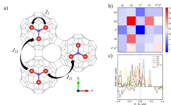
Fig. 3 (a) Schematic representation of intra/intermolecular magnetic interactions in the  $V_3N@C_{80}$  network. (b) Orbital contribution to  $J_{21}$  from interacting first neighbor V atoms. (c) PDOS of d orbitals of V atoms in  $J_{21}$  and C atoms in linking moieties of  $V_3N@C_{80}$ .
