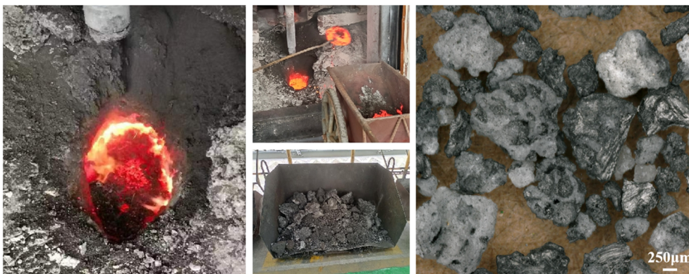
Fig. 1 Removal, temporary storage, and microstructural characterization of carbon dross in an aluminum electrolysis plant in China.
