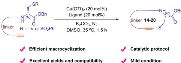
**Cu-catalyzed alkynylation of thiosulfonate-based peptide: an efficient approach to S-alkynyl-containing cyclic peptides**
