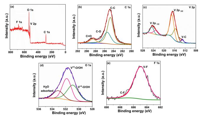
Fig. 2 XPS analysis of the V<sub>2</sub>CT<sub>x</sub> MXene: (a) total survey, (b) C 1s, (c) V 2p, (d) O 1s, and (e) F 1s spectra.
