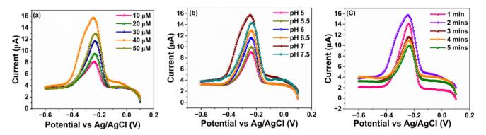
Fig. 4 Square wave voltammograms (SWV) obtained at (a) different HER-2 aptamer concentrations, (b) effect of varying pH levels within the range of 5 to 7.5 on the hybridization of 100 µM recombinant protein, and (c) influence of incubation time on the response of 100 µM HER-2 recombinant protein.
