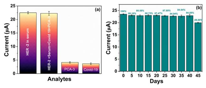
Fig. 6 (a) Inference analysis of the HER-2 aptasensor in the presence of various analytes. (b) Shelf-life evaluation of the developed sensor over 40 days.
