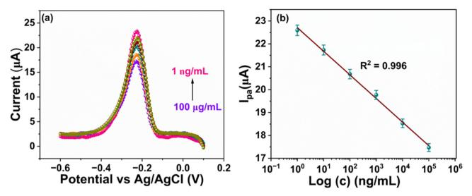
Fig. 5 (a) Square wave voltammetric profiles at various concentrations of the recombinant HER-2 protein ranging from 1 ng mL<sup>-1</sup> to 100  $\mu$ g mL<sup>-1</sup>. (b) Sensor calibration graph was achieved at 0.22 V (–220 mV), showing a linear correlation between the peak current ( $I_{pa}$ ) and the HER-2 recombinant protein concentrations.
