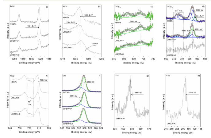
Fig. 5 High-resolution XPS spectra of the HEOFe, LiHEOFeF, and LiHEOFeCl compounds showing the signals corresponding to (a) Zn 2p, (b) Mg 1s, (c) Co 2p<sub>1/2</sub>, (d) Cu 2p<sub>3/2</sub>, (e) Fe 2p, (f) O 1s, (g) F 1s and (h) Cl 2p.
