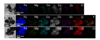
Fig. 3 (S)TFM micrograph of the synthesized (a) HFOFe (b) LiHFOFeF and (c) LiHEOFeCl samples with the corresponding elemental maps determined by EDS.
