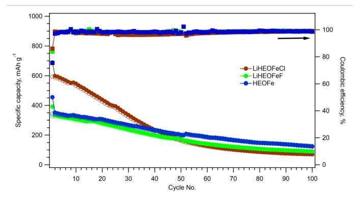
Fig. 7 Galvanostatic chronopotentiometry at 1C rate for HEOFe (blue circles), LiHEOFeCl (brown circles), and LiHEOFeF (green circles). The charge capacity within charging is marked with full circles and the charging capacity within discharging with empty circles. The corresponding coulombic efficiencies for HEOFe, LiHEOFeCl, and LiHEOFeF are depicted by squares of the same color coding.
