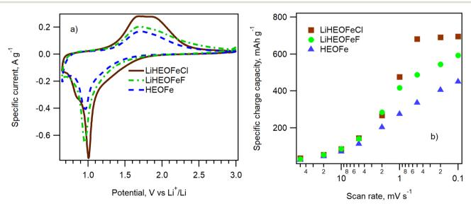
Fig. 6 (a) Cyclic voltammograms measured on 2032-coin cells containing LiHEOFeCl, LiHEOFeF, and HEOFe with a scan rate of 0.1 mV s<sup>-1</sup>. (b) The scan-rate dependence of the charge capacities calculated from the discharge branch of the cyclic voltammogram on the scan rate for HEOFe (blue triangles), LiHEOFeCl (brown squares), and LiHEOFeF (green circles).
