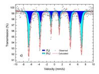
Fig. 4 The room-temperature <sup>57</sup>Fe Mössbauer spectra of (a) HEOFe, (b) LiHEOFeF, and (c) LiHEOFeCl. The dark blue and light blue spectra correspond to tetrahedrally (Td) and octahedrally [Oh] coordinated iron cations, respectively.
