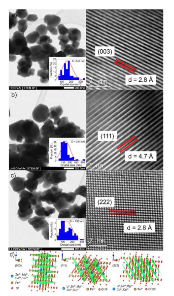
Fig. 2 (S)TEM and HR-TEM micrographs of (a) HEOFe, (b) LiHEOFeF, and (c) LiHEOFeCl synthesized samples. Insets show the particle size distribution. Interplanar distances, d, correspond to those determined from eqn (5). (d) Idealized spinel structure of the investigated samples. Particular crystal planes for HEOFe (003), LiHEOFeF (111), and LiHEOFeCl (222) are highlighted.
