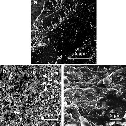
Fig. 1 Scanning electron microscopic images of (a) Ag nanoparticles, (b) hBN powder and (c) as-prepared BNOH.
