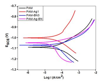
Fig. 7 Potentiodynamic polarization curve of PAM, PAM-Ag1, PAM-BN3 and PAM-Ag-BN hydrogels.
