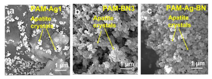
Fig. 9 Surface morphology of (a) PAM-Ag1, (b) PAM-BN3 and (c) PAM-Ag-BN hydrogels showing apatite formation.
