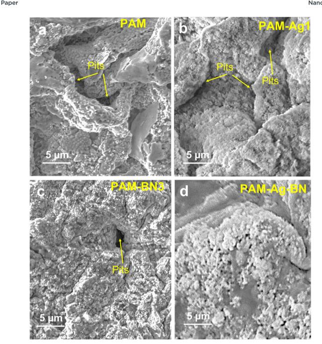
Fig. 8 Scanning electron microscopic images of the top surface of (a) PAM, (b) PAM-Ag1, (c) PAM-BN3 and (d) PAM-Ag-BN hydrogels after corrosion testing.
