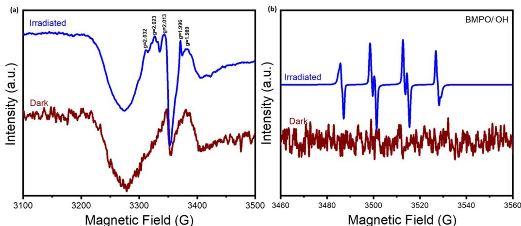
Fig. 8 (a) EPR spectra of the Au SA/TiO<sub>2</sub> sample under subsequential dark and light conditions at 90 K. (b) The spin trapping tests of Au SA/TiO<sub>2</sub> for detecting hydroxyl (<sup>•</sup>OH) radical formation by using 5-*tert*-butoxycarbonyl-5-methyl-1-pyrroline-*N*-oxide (BMPO) as a spin trapping agent.
