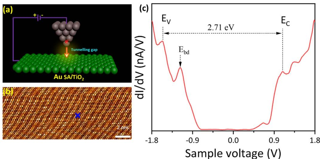
Fig. 4 (a) The schematic illustration of scanning tunneling microscopy (STM) analysis, (b) and (c) topography STM image and tunneling spectroscopy of the Au SA/TiO<sub>2</sub> sample recorded from the green cross in (b). Tunneling conditions:  $V_{\text{sample}} = 1.8$  V,  $I_t = 200$  pA. The valence and conduction band edges of Au SA/TiO<sub>2</sub> are indicated by vertical segments, labeled as  $E_V$  and  $E_C$ . The  $E_{bd}$  stands for bright defects in the TiO<sub>2</sub> structure.
