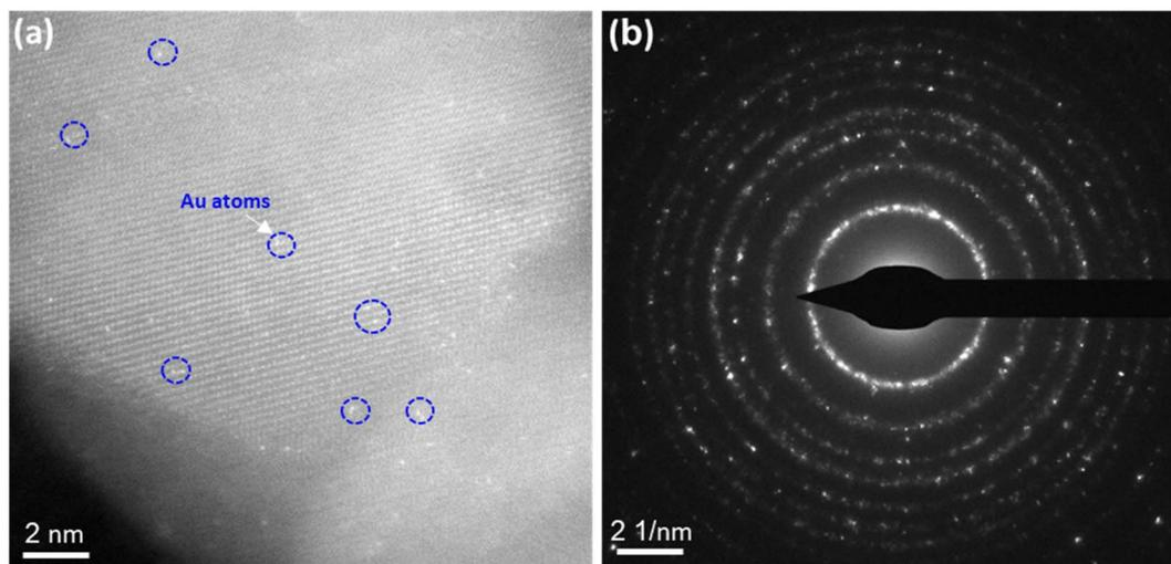
Fig. 3 The HR-TEM image and SAED images of Au SA/TiO<sub>2</sub> powder, respectively (a) and (b). The bright spots in (a) indicate Au single atoms (SA) over the TiO<sub>2</sub> matrix.
