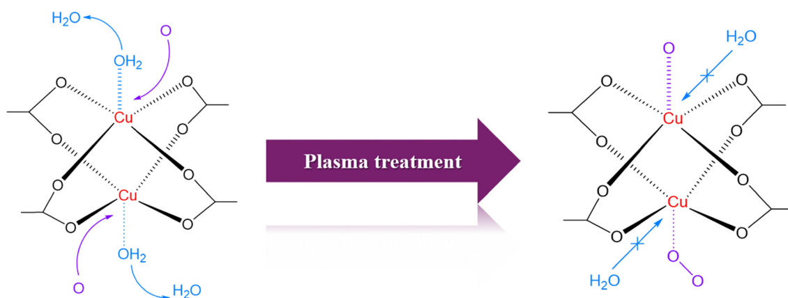
Fig. 7 Proposed \text{O}_2 plasma treatment mechanism of pore activation and protection. Reproduced from ref. 71 with permission from RSC, copyright 2017.
