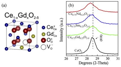
Fig. 7 (a) Crystal structure of  $Ce_{1-x}Gd_xO_{2-\delta}$ ; <sup>140</sup> (b) XRD patterns of  $Ce_{0.8}Sm_{0.25}O_{2-\delta}$ ,  $Ce_{0.8}Gd_{0.25}O_{2-\delta}$  and  $Ce_{0.8}Nd_{0.25}O_{2-\delta}$ . Reproduced from ref. 140 with permission from [Elsevier], copyright [2017]. Reproduced from ref. 141 with permission from [Elsevier], copyright [2017]
