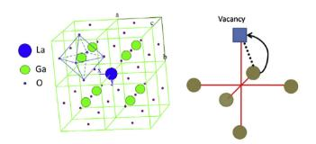
Fig. 9 The cubic ABO<sub>3</sub> perovskite structure, and the path of oxygen ions migration along BO<sub>6</sub> octahedron edge. 184 Reproduced from ref. 184 with permission from [Elsevier], copyright [1995]
