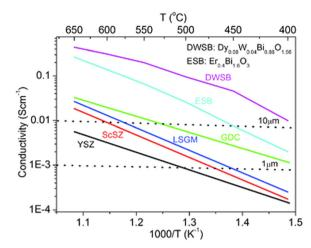
Fig. 6 Conductivities of electrolyte materials at different operating temperatures. The horizontal dashed line indicated the conductivity requirement to achieve ASR  $< 0.1\,\Omega$  cm $^{-1}$  at the thickness of 1  $\mu$ m and 10  $\mu$ m. $^{118}$ Reproduced from ref. 118 with permission from [Royal Society of Chemistry], copyright [2016]
