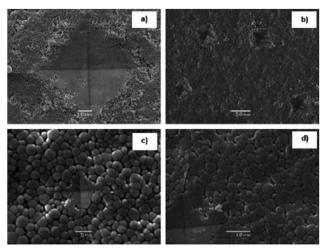
Fig. 21 The sample of Ce<sub>0.9</sub>Gd<sub>0.1</sub>O<sub>1.95</sub> of Pyramid-shaped Vickers indentation marks on tape sintered at (a) 1300, (b) 1400 °C/2 h, (c) and (d) indentation imprint and emanated crack on the tapes sintered at 1500  $^{\circ}\text{C}$  2  $\text{h}^{-1.358}$ Reproduced from ref. 358 with permission from [Wiley], copyright [2013].
