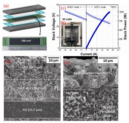
Fig. 23 (a) Schematic diagram of reversible SOC with repeating cell units; (b) photograph of 1 kW class stack; (c) I-V curves of both SOEC and SOFC mode for 30-cell stack at 700 °C; (d) and (e) cross-section SEM image of the cell area and Ag glass interconnector. 369 Reproduced from ref. 369 with permission from [Elsevier], copyright [2022].
