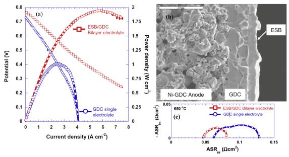
Fig. 19 /-V characteristics of fuel cell samples with single layer GDC and bilayer ESB/GDC electrolyte at 650 °C using 90 sccm of air and wet hydrogen. (b) SEM micrograph of the cross-section of ESB/GDC bilayer electrolyte with anode support. (c) Impedance spectra of the GDC and ESB/GDC electrolyte. 349 Reproduced from ref. 349 with permission from [Elsevier], copyright [2009].
