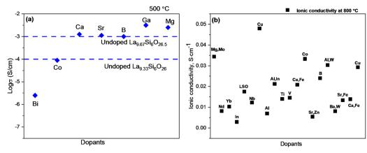
Fig. 10 (a) Comparison of conductivities of different dopants at a constant level of oxygen excess at 500 °C; (b) ionic conductivity of different dopants
