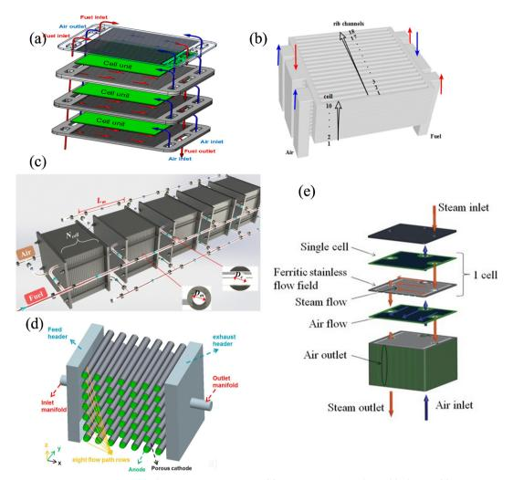
Fig. 22 (a) The schematic diagram of a planer SOFC stack with three cell unit; (b) 3D structure of the 10-cell SOFC stack; (c) the schematic diagram of an integrated muti-SOFC stack and (d) tubular SOFC stack with anode support and (e) 20-cell SOE stack. 362,363,365,366,368 Reproduced from ref. 362 with permission from [MDPI], copyright [2018]. Reproduced from ref. 363 with permission from [Elsevier], copyright [2023]. Reproduced from ref. 365 with permission from [Elsevier], copyright [2018].
