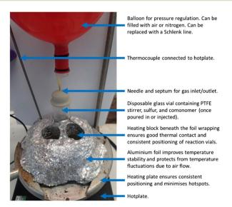
A recommended inverse vulcanisation bulk polymerisation set up
