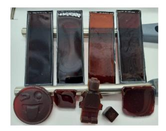
Fig. 8 Inverse vulcanised polymers that have been moulded into various shapes and dimensions, by pouring the pre-polymer into a mould and then curing the pre-polymer until it is shape persistent. Fully reacted inverse vulcanised polymers of low  $T_{\rm g}$  can also be melt processed in this fashion.
