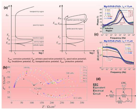
Fig. 17 (a) Schematic of polarization curves. Reproduced from ref. 302 with permission from Elsevier, copyright 2018. (b) In situ Nyquist plots of the Mg electrode in  $Na_2SO_4$  electrolytes. Reproduced from ref. 306 with permission from Elsevier, copyright 2019. (c) Bode phase and Bode |Z| plots of the Mg-0.6%Si-2%Zn alloys. (d) Equivalent electrical circuit. Reproduced from ref. 307 with permission from Elsevier, copyright 2024.
