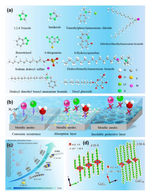
Fig. 13 (a) Molecular structures of commonly used organic inhibitors. (b) Schematic of the corrosion inhibition mechanism of organic inhibitors. (c) HOMO energy level of different molecules. Reproduced from ref. 212 with permission from Elsevier, copyright 2024. (d) Channel size illustration of CuC<sub>7</sub> and CuC<sub>15</sub> with different alkyl chain lengths. Reproduced from ref. 213 with permission from the Royal Society of Chemistry, copyright 2024.
