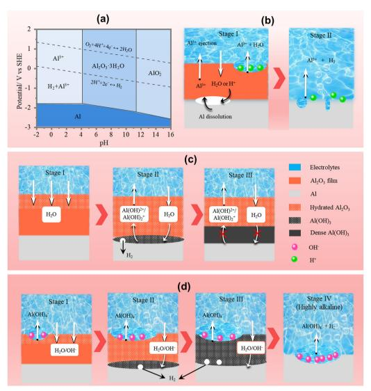
Fig. 3 (a) Pourbaix diagram of Al-H<sub>2</sub>O at 25 °C. Illustration of the corrosion mechanism of the Al anode in (b) acidic electrolytes, (c) neutral electrolytes, and (d) alkaline electrolytes.
