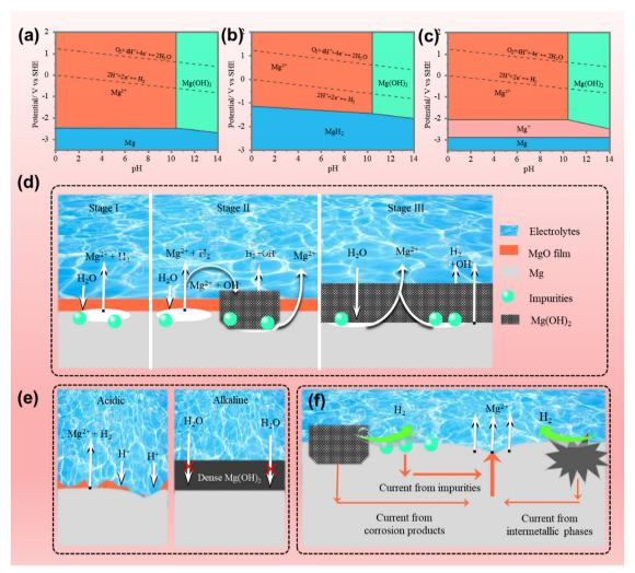
Fig. 4 Pourbaix diagrams of  $Mg-H_2O$  at 25 °C (a) without  $Mg^+$  and  $MgH_2$ , (b) in the presence of  $MgH_2$ , and (c) in the presence of  $Mg^+$ . Corrosion mechanism of Mg (d) in neutral electrolytes, and (e) in acidic and alkaline electrolytes. (f) Galvanic corrosion mechanism of Mg.
