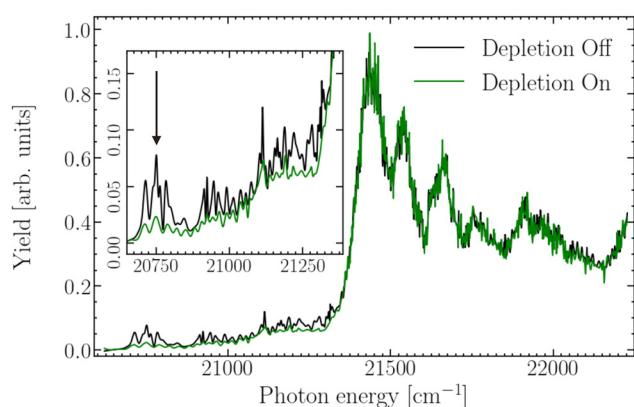
**Fig. 4** Prompt action-absorption spectrum without a depletion laser (black), and with a depletion laser (green) being applied. The arrow at  $20747\text{ cm}^{-1}$  indicates the photon energy of the depleting photons.
