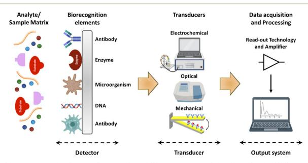
Fig. 33 Schematic representation of biosensor. (Reproduced from ref. 251 with permission from Springer Nature, Copyright 2023.)
