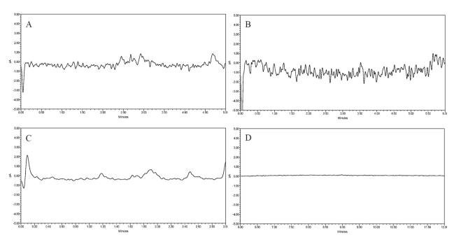
Fig. 3 Comparison of the baseline results of different HILIC chromatographic columns. (A) Agilent ZORBAX-NH2 (4.6 mm × 250 mm, 5 μm), (B) Welch Ultimate XB-NH<sub>2</sub> (4.6 mm × 250 mm, 5 μm), (C) waters XBridge BEH amide (4.6 mm × 150 mm, 3.5 μm), (D) Agilent InfinityLab Poroshell 120 HILIC (4.6 mm  $\times$  150 mm, 2.7  $\mu$ m)
