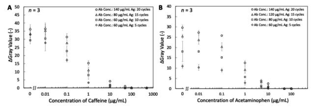
Fig. 9 Different dynamic response ranges for target analytes in artificial urine matrix: caffeine (A), acetaminophen (B) achieved by adjusting the amount of labeled antibody deposited on conjugate pads and inkjet printing cycles of BSA-conjugates on the NC membrane; error bars represent one standard deviation from the mean (n = 3).
