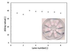
Fig. 3 Signal intensities recorded for each individual LFIA lane in a single device of type B after application of a blank sample.
