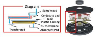
Fig. 2 Schematic diagram showing sample liquid flow path through a single assay lane of LFIA device type B.
