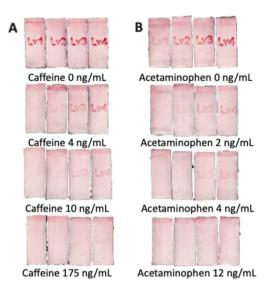
Fig. 10 Text-displaying results for the semi-quantitative detection of (A) caffeine = 0, 4, 10, 175 ng mL $^{-1}$ , (B) acetaminophen = 0, 2, 4, 12 ng mL $^{-1}$  in artificial urine samples. The figure shows a zoom-in to each LFIA lane on a single device; brightness, contrast and saturation have been modified to improve visibility; the unmodified originals of overall devices are shown in Fig. S6.†
