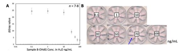
Fig. 4 (A) 8-OHdG concentration-dependent response of assays performed with device type B (8-OHdG = 0.1, 1, 10, 30, 50, 70, 100 ng mL $^{-1}$ ), and (B) color scans of corresponding devices; error bars represent one standard deviation from the mean (n = 7 or 8); blue arrow in (B) marks an LFIA lane with irregular flow behavior.
