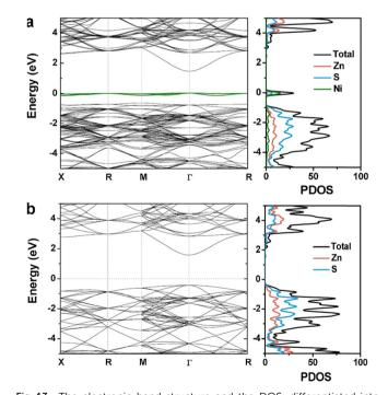
Fig. 13 The electronic band structure and the DOS; differentiated into total and partial. (a) ZnS that is 2.7% doped with Ni and (b) undoped ZnS. $^{52}$
