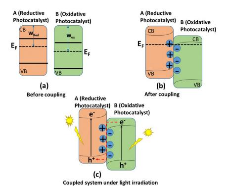
Fig. 9 The mechanism of direct Z-scheme photocatalyst production using oxidative and reductive semiconductors, showing the band structures (a) before and (b) after coupling. (c) The band structure of a linked system under light irradiation. The Fermi energy level is denoted by the symbol  $E_F$ .
