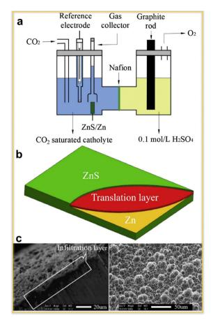
**Fig. 3** (a) An organic electrolyte-based two-compartment electrolysis cell, (b) an infiltration layer schematic and (c) a scanning electron micrograph of a ZnS electrode. <sup>75</sup>
