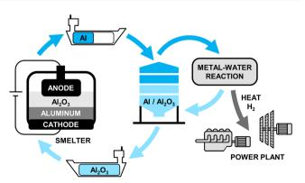
Fig. 2 Aluminum fuel cycle consisting of four main components: aluminum production, transportation, storage, and power generation.
