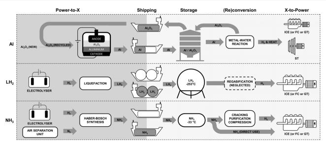
Fig. 6 Overview the carbon-free energy carrier pathways studied. The darker grey portion on the left corresponds to the equipment and processes needed at the production site, prior to shipping. The rest is needed at the remote mine site
