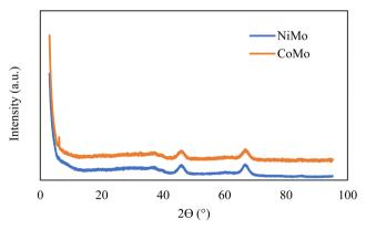
Fig. 3 XRD results of hydrotreating catalysts.
