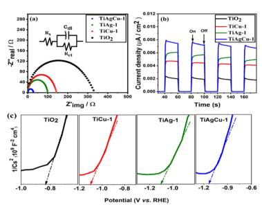
Fig. 4 (a) Nyquist plots, (b) transient photocurrent responses under light illumination conditions, and (c) Mott-Schottky plot of TiO2, TiAg-1, TiCu-1, and TiAgCu-1. The electrochemical experiments were carried out in 0.5 M Na<sub>2</sub>SO<sub>4</sub> (pH = 7.5) at a potential of 1.23 V (vs. NHE)
