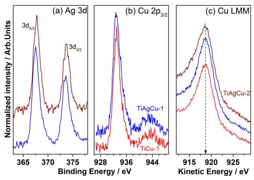
Fig. 5 XPS core level spectra recorded for (a) Ag 3d and (b) Cu 2p<sub>3/2</sub> core levels, and (c) X-ray initiated Auger electron spectra recorded for Cu-L<sub>3</sub>M<sub>45</sub>M<sub>45</sub> transition for TiCu-1, TiAgCu-1 and TiAgCu-2 nanocomposites. Different colours were used for different compositions, namely, TiCu-1 (red), TiAgCu-1 (blue), and TiAgCu-2 (brown).
