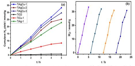
Fig. 7 (a) Time on stream dependence of solar hydrogen production of the mesoporous TiO2, TiAg-1, TiCu-1 and TiAgCu nanocomposites (in thin film form) from solar hydrogen evolution. (b) Solar hydrogen production as a function of time with repeated cycles of operation for TiAgCu-1 in direct sunlight.
