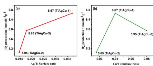
(a) Variation of rate of hydrogen production with Aq/Ti surface ratio. (b) Variation of rate of hydrogen evolution with Cu/Ti surface ratio.
