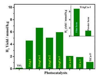
Fig. 6 Photocatalytic H<sub>2</sub> production activity of mesoporous TiO<sub>2</sub>, Ag/ TiO<sub>2</sub>, Cu/TiO<sub>2</sub> and Ag-Cu/TiO<sub>2</sub> nanocomposites, measured in thin film form under direct sunlight. Inset shows a comparison of the solar hydrogen generation activity for the thin film and powder catalysts of TiAgCu-1.
