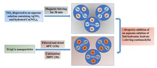
Scheme 1 Schematic illustration of the synthesis of mesoporous Ag-Cu/TiO2 nanocomposites.
