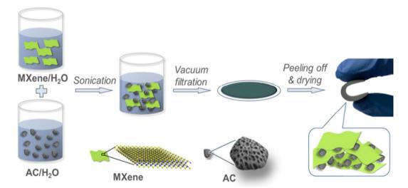
Fig. 15 Schematic showing the process for creating MXene-bonded AC films, which involved dispersing AC particles and MXene flakes in water, followed by a vacuum-assisted filteration, peeling-off of the excess material, and drying. Reprinted with permission from ref. 87. Copyright 2018, American Chemical Society
