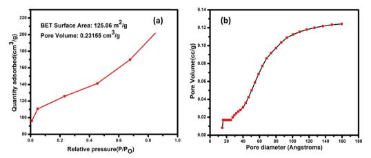
(a) BET adsorption isotherm and the (b) pore size distribution curve.
