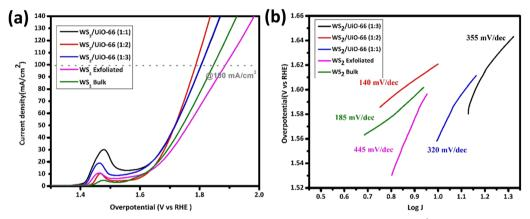
Fig. 6 (a) LSV OER curves of bulk WS<sub>2</sub>, exfoliated WS<sub>2</sub>, WS<sub>2</sub>@UiO-66(1:1, 1:2, 1:3) at a scan rate of 10 mV s<sup>-1</sup> in 1.0 M KOH. (b) Corresponding Tafel plots of bulk WS<sub>2</sub>, exfoliated WS<sub>2</sub> and WS<sub>2</sub>@UiO-66(1:1, 1:2, 1:3).
