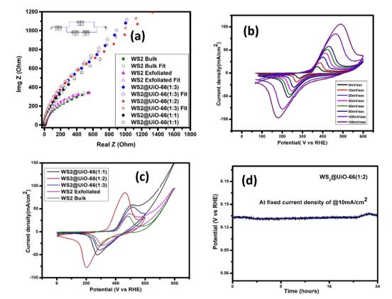
Fig. 7 (a) EIS Nyquist plots of all the prepared hybrids with fitted curves. (b) CV of WS2@UiO-66(1:2) at different scan rates. (c) CV of all the prepared hybrids at a scan rate of 50 mV s<sup>-1</sup>. (d) Stability test at a fixed current density of 10 mA cm<sup>-2</sup>.
