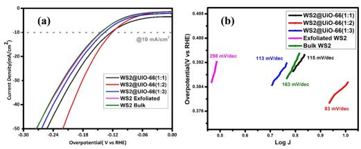
Fig. 5 (a) LSV HER curves of bulk WS<sub>2</sub>, exfoliated WS<sub>2</sub>, and WS<sub>2</sub>@UiO-66(1:1, 1:2, and 1:3) at a scan rate of 10 mV s<sup>-1</sup> in 1.0 M KOH. (b) Corresponding Tafel plots of bulk WS<sub>2</sub>, exfoliated WS<sub>2</sub> and WS<sub>2</sub>@UiO-66(1:1, 1:2, 1:3).
