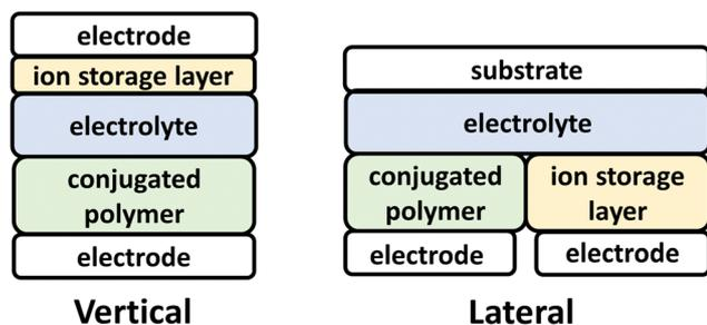
Fig. 3 Vertical (left) and lateral (right) ECD architectures.
