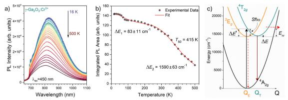
Fig. 8 (a) Temperature dependence of the PL emission spectra of γ-Ga<sub>2</sub>O<sub>3</sub>:Cr<sup>3+</sup> NCs from 16 to 500 K (7). (b) Temperature dependence of the integrated PL intensity (black dots) and fit (red curve). (c) Configurational coordinate diagram constructed by using eqn (5)-(7).
