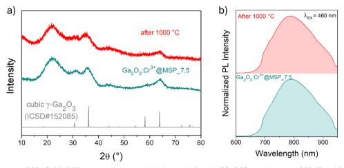
Fig. 5 Stability tests up to 1000 °C. (a) XRPD pattern of the sample before and after the TG-DSC analysis up to 1000 °C and (b) the corresponding normalized PL spectra obtained after excitation at 460 nm.
