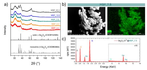
Fig. 2 (a) XRPD patterns of the samples with increasing pore size of the mesopores of the MSPs where the Ga<sub>2</sub>O<sub>3</sub> NCs were grown. (b) Representative secondary electron-SEM image and corresponding EDX elemental map of Ga and (c) EDX spectrum of the Ga<sub>2</sub>O<sub>3</sub>:Cr<sup>3+</sup>@MSP\_7.5 sample.
