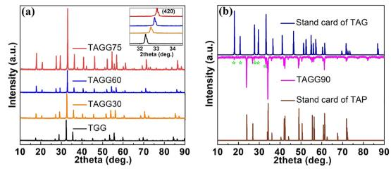
Fig. 2 (a) Powder XRD patterns of TAGG ( $x \le 0.75$ ) crystals. The inset shows the right shift of the enlarged (420) diffraction peaks. (b) XRD patterns of TAGG90 as well as TAG and TAP for comparison.
