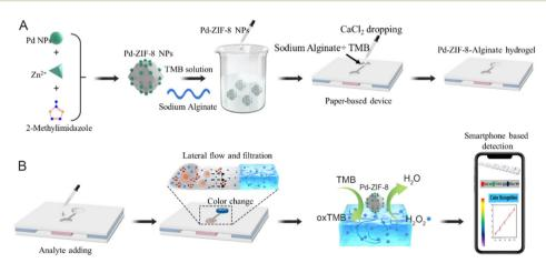
Scheme 1 Schematic illustration of PAD hydrogel-based separation-free device for H<sub>2</sub>O<sub>2</sub> detection by a smartphone.
