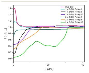
Fig. 3 Probe approach curves measured at various stages of cycling at 1.7 mA cm<sup>-2</sup>. Measurements were recorded after the first, fifth, and tenth plating for zinc-metal anodes in 1 M and 2 M ZnSO<sub>4</sub>. An increase in tip current beyond l = 1 denotes positive feedback, and a decrease in tip current below l = 1 denotes negative feedback. A charge of 1.7 mA h cm<sup>-2</sup> (4 mg cm<sup>-2</sup> zinc) was passed per plating/stripping cycle.
