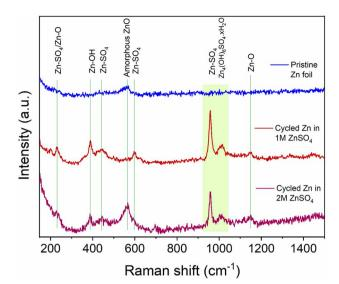
Fig. 10 Comparison of Raman spectra of bare and cycled Zn electrodes. The assignments of key bands are made based on reference samples (Fig. S41-S45†). The electrodes were cycled for 40 h (20 cycles) in 1 M and 2 M ZnSO<sub>4</sub> electrolytes with a Celgard 3501 polymer separator. Samples were washed with distilled water prior to measurement
