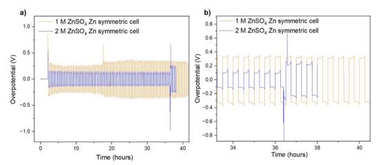
Fig. 8 (a) Voltage trace (E vs. t) of successive galvanostatic cycling of a total of 2.75 mA h cm<sup>-2</sup> of zinc at 11 mA cm<sup>-2</sup> (4C) in zinc symmetric cell with 2 M ZnSO₄ aqueous electrolyte, glass fibre separator. (b) Magnification of voltage trace (E vs. t) at the soft short formation.
