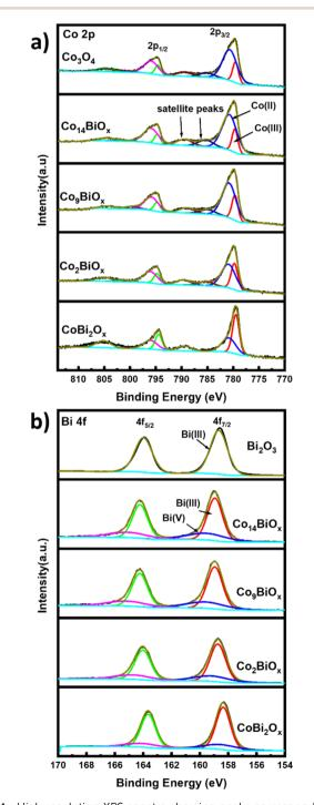
Fig. 4 High resolution XPS spectra showing peaks corresponding to (a) Co 2p and (b) Bi 4f of Co<sub>3</sub>O<sub>4</sub>, Co<sub>14</sub>BiO<sub>x</sub>, Co<sub>9</sub>BiO<sub>x</sub>, Co<sub>2</sub>BiO<sub>x</sub>, CoBi<sub>2</sub>O<sub>x</sub>, and Bi<sub>2</sub>O<sub>3</sub> catalysts.
