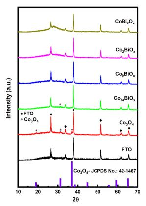
Fig. 2 XRD patterns of FTO substrate and the different catalysts synthesized *in situ* on FTO substrates, namely  $Co_3O_4$ ,  $Co_{14}BiO_x$ ,  $Co_2BiO_x$ , and  $CoBi_2O_x$ . The XRD pattern of  $Co_3O_4$  obtained from the JCPDS database is included for reference.
