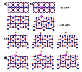
Fig. 6 Top view and side view images of (a) Co<sub>3</sub>O<sub>4</sub>(100) surface and (b) Bi-doped Co<sub>3</sub>O<sub>4</sub>(100) surface. Red: oxygen, blue: cobalt, and purple: bismuth. Optimized structures of (c) Co<sub>3</sub>O<sub>4</sub>(100) surface and (d) Bidoped Co<sub>3</sub>O<sub>4</sub>(100) surface, with both showing surface-adsorbed \*OH, \*O, and \*OOH intermediates.
