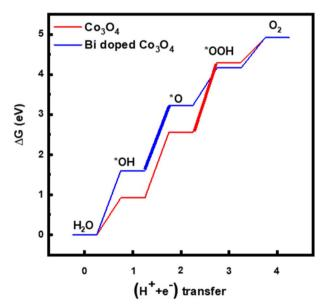
Fig. 7 Diagrams showing calculated free energy changes of OER on the surface of Co<sub>3</sub>O<sub>4</sub>(100) and Bi-doped Co<sub>3</sub>O<sub>4</sub>.
