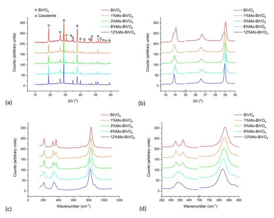
Fig. 2 (a) XRD patterns, (b) close-up view of select peaks in XRD patterns, (c) Raman spectra and (d) close-up view of select peaks in Raman patterns of BiVO<sub>4</sub> and all Mo-doped BiVO<sub>4</sub> samples.
