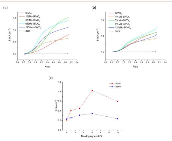
Fig. 6 Current voltage (JV) curves for BiVO<sub>4</sub> and all Mo-doped BiVO<sub>4</sub> samples measured with (a) front irradiation and (b) back irradiation. (c) The photocurrent densities observed at 1.23 V<sub>RHE</sub> for both front and back irradiation as a function of Mo precursor doping level (%) of BiVO<sub>4</sub> and all Mo-doped BiVO<sub>4</sub> samples. Samples were measured in 0.1 M phosphate buffer (pH = 7) using 400 nm light ( $\sim$ 8.5 mW cm<sup>-2</sup>).
