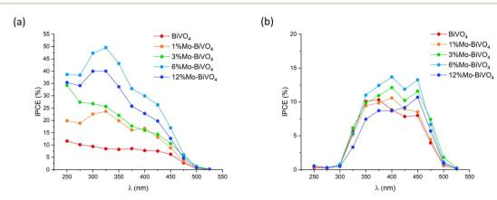
Fig. 7 Incident photon to current efficiency (IPCE) curves for BiVO<sub>4</sub> and all Mo-doped BiVO<sub>4</sub> samples measured with (a) front irradiation and (b) back irradiation. Samples were measured in 0.1 M phosphate buffer (pH = 7) at 1.23  $V_{RHF}$ .
