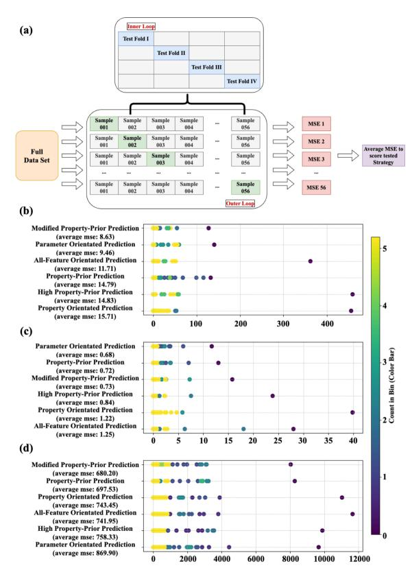
Fig. 8 (a) Evaluation of the ML strategy based on LOOCV and NCV, and visualized performance of Mean Squared Error (MSE) in predicting (b) photocatalytic NO conversion, (c) photocatalytic  $NO_x$  conversion and (d) photocatalytic  $NO_2$  selectivity in 56 NCV cycles for each ML strategy, where colours represent the number of times the MSE falls within this range.
