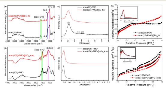
Fig. 1 FT-IR spectra of (a) acac(20)-PMO and (d) acac(100)-PMO; XRD patterns of (b) acac(20)-PMO and (e) acac(100)-PMO; N<sub>2</sub> adsorptiondesorption isotherms and pore size distributions of (c) acac(20)-PMO and (f) acac(100)-PMO.
