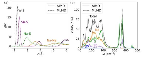
Fig. 8 (a) g(r) and (b) VDOS for W-doped Na<sub>2.94</sub>Sb<sub>0.94</sub>W<sub>0.06</sub>S<sub>4</sub> as computed from AIMD and MLMD
