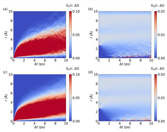
Fig. 4 Spatiotemporal correlations of Ag<sup>+</sup> ion migration in AgI: (a) and (c) visualize the self-part,  $G_s(r, \Delta t)$ , of the van Hove correlation extracted from AIMD and MLMD simulations, respectively. Panels (b) and (d) visualize the distinctive part,  $G_d(r, \Delta t)$ , from AIMD and MLMD simulations, respectively. MLMD data were averaged across 5 independent trajectories.
