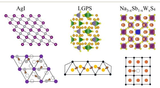
Fig. 1 Schematic representation of the solid-state ionic conductors investigated in this work: (Left) AgI, with Ag in silver and I in purple; (mid)  $Li_{10}GeP_2S_{12}$  (LGPS) with Li in bright orange, Ge in grey, P in green and S in yellow; (right)  $Na_{3-x}Sb_{1-x}W_xS_4$  with Na in dark orange, W in blue, Sb in purple and S in yellow. The ion-conduction mechanisms of each system are sketched in the lower panels.
