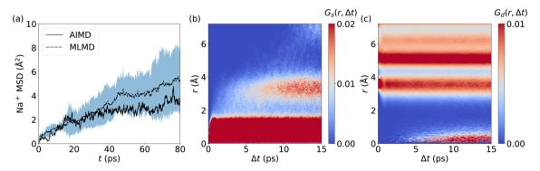
Fig. 9 (a) MSD of Na<sup>+</sup> ions in Na<sub>2.94</sub>Sb<sub>0.94</sub>W<sub>0.06</sub>S<sub>4</sub> as a function of t, with the dashed line being the average of 5 MLMD runs and the blue-shaded region the standard deviation. Spatiotemporal correlations of Na<sup>+</sup> ion migration: Panels (b) and (c) visualize  $G_s(r, \Delta t)$  and  $G_d(r, \Delta t)$ , respectively. MLMD data were averaged across 5 independent trajectories.
