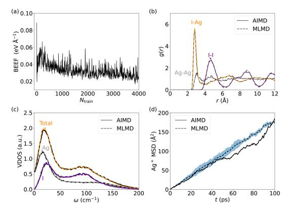
Fig. 2 (a) Bayesian error estimate of forces (BEEF) as function of the number of training steps,  $N_{\text{train}}$ , during training of the MLFF for Agl. Panels (b) and (c) visualize the atomic pair correlation function, g(r), and the vibrational density of states (VDOS), respectively. In panel (d) the mean square displacement (MSD) of Ag<sup>+</sup> ions is shown as a function of time, t, with the dashed line being the average of 5 MLMD runs and the blue-shaded region the standard deviation.
