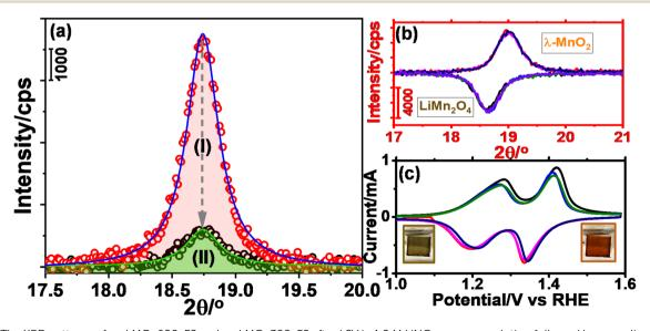
Fig. 5 (a) The XRD patterns of m-LMO-600-F2 and m-LMO-300-F2 after LSV in 1.0 M LiNO $_3$  aqueous solution followed by annealing at 600 °C (relative area under diffraction lines (I) 100 and (II) 16.3) and (b) the XRD patterns of m-LMO-300-F2 after LSV from 1.0 to 1.6 V and in reverse cycles from 1.6 to 1.0 V (repeated 3 times), and (c) 3 CVs of the m-LMO-300-F2 electrode (insets show the color of the electrodes on each side of the potential window).
