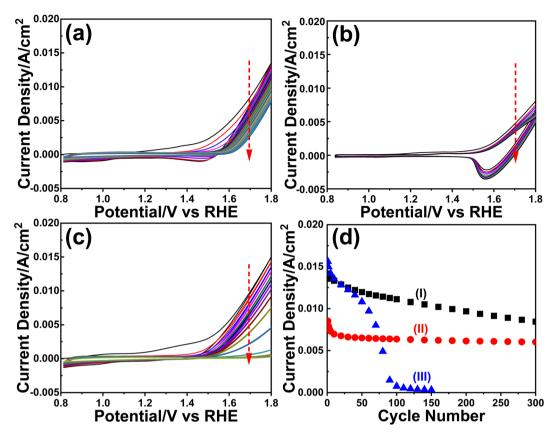
Fig. 6 The CV curves (50 mV s $^{-1}$  scan rate) of the m-LMO-300-F2 electrode in (a) 1.0 M KOH and (b) 1.0 M LiOH and (c) the CV curves (50 mV s $^{-1}$ scan rate) of the m-Mn<sub>3</sub>O<sub>4</sub>-300-F2 electrode in 1.0 M KOH (red arrows indicate the cycling order). (d) Plot of current density values at 1.8 V versus CV cycle numbers of the electrodes, (I) m-LMO-300-F2 in 1.0 M KOH, (II) m-LMO-300-F2 in 1.0 M LiOH, and (III) m-Mn<sub>3</sub>O<sub>4</sub>-300-F2 in 1.0 M КОН.
