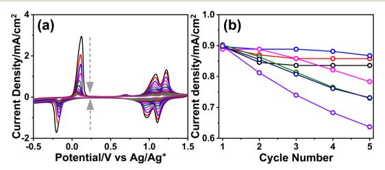
Fig. 3 (a) The CV curves of the m-LMO-300-F2 electrode in 1.0 M LiClO<sub>4</sub> acetonitrile solution (arrows represent the cycle order) and (b) the plot of the current density at 1.4 V of the m-LMO-300-F2 electrode versus cycle numbers in 1.0 M LiNO<sub>3</sub> aqueous solution with respect to the starting potential of a forward sweep in the CV curves, where black: 0.75 V, red: 0.45 V, blue: 0.15 V, pink: 0.05 V, green: -0.05 V, dark blue: -0.15 V, and purple: -0.2 V.
