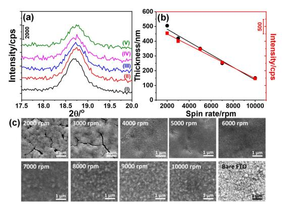
Fig. 1 (a) The XRD patterns of m-LMO-300-F# films between 17.5 and 20.0°, 2θ, coated at (I) 2000, (II) 3000, (III) 5000, (IV) 7000 and (V) 10 000 rpm, (b) the plots of the film thickness and X-ray intensity of the m-LMO-300-F# films versus spin-rate (black dots from SEM images and red squares are (111) diffraction line intensity values at 18.7°,  $2\theta$ ), and (c) the SEM images (top view) of the thin films at indicated spin-rates.
