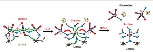
Scheme 1 Electrode degradation mechanism of LiMn<sub>2</sub>O<sub>4</sub> electrodes during the OER.
