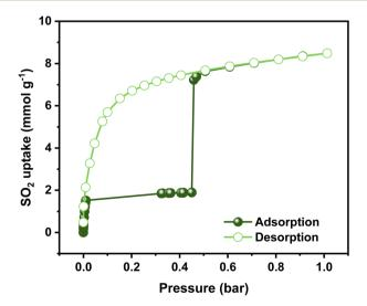
Fig. 2 Experimental  $SO_2$  adsorption—desorption isotherm of an activated NiBDP sample (filled green circles = adsorption; open green circles = desorption) at 298 K up to 1 bar.
