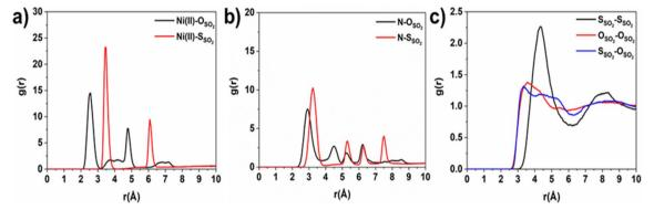
Fig. 6 Intermolecular radial pair distribution functions of NiBDP-0H<sub>2</sub>O MOF atoms and adsorbed SO<sub>2</sub> molecules were calculated at P = 0.10 bar (a and b), and guest  $SO_2-SO_2$  (c) was calculated at P=0.50 bar.
