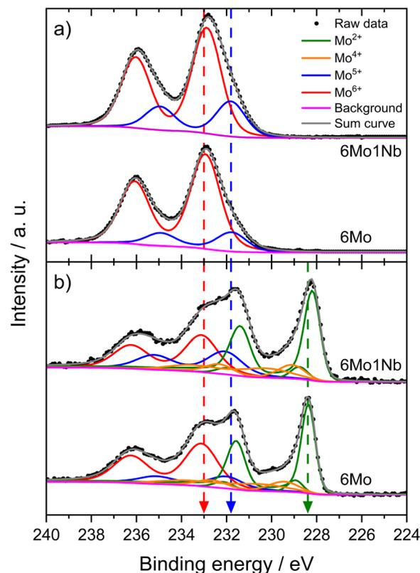
Fig. 6 Intensity-normalized XP spectra for the Mo 3d core level of fresh (a) and spent (b) 6Mo/HZSM-5 and 6Mo1Nb/HZSM-5 catalysts. Reaction conditions: 700 °C, 300 mg catalyst, 90% CH<sub>4</sub> + 10% N<sub>2</sub>, 3200 SCC g<sub>cat</sub><sup>-1</sup> h<sup>-1</sup>, 1 atm, 6 h. Dashed lines were added as a visual guide.
