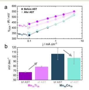
Fig. 5 Tafel analysis of  $Mn_{70}Ti_{30}O_x$  and  $Mn_{90}Co_{10}O_x$ . (a) Tafel plot for both samples before and after the AST. Standard deviation calculated from duplicates. (b) Tafel slopes calculated from (a) before and after the AST.
