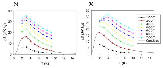
Fig. 8 Magnetic entropy change,  $-\Delta S_{m}$ , for 1 grafted on a TSP functionalized Si wafer, 1Si, with the wafer parallel (a) and perpendicular (b) to the SQUD magnetic field. The solid line is a mathematical fit to a logarithmic peak function.
