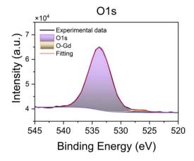
Fig. 3 HAXPES spectra for the Gd  $2p_{1/2}$  and the O 1s core levels of 1Si.
