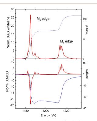
Fig. 6 Normalized, background-subtracted XAS and XMCD spectra at the M<sub>4.5</sub> edges of Gd measured at 3.4 K and 6 T, and the associated integrated signals (right scale).
