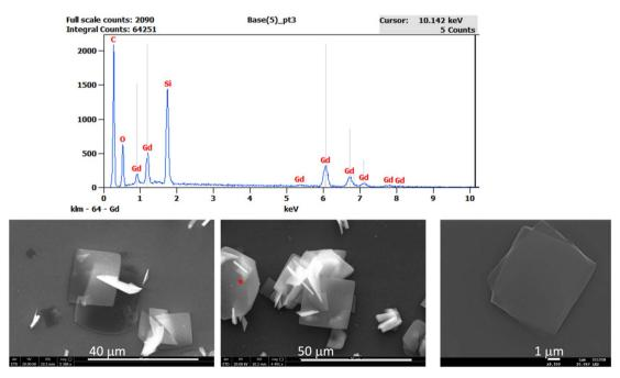
Fig. 2 SEM images for **1S**i (48 h deposition time) showing the growth of microcrystals form the functionalized Si. The EDS analysis corresponds to the flake with the red asterisk on the central image.
