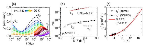
Fig. 5 (a) Imaginary component of the ac susceptibility as a function of the frequency,  $\chi''(f)$ , of complex 1 at  $\mu_0H=0.2$  T and different temperatures ranging from 1.8 K to 20 K; (b) magnetic relaxation time as a function of the inverse temperature (1/T) at  $\mu_0H=0.2$  T; (c) temperature dependence of  $\tau_2^{-1}(T)$ , and a fit to a power law  $\tau_2^{-1}=KT^2$ , with K=235 s<sup>-1</sup> K<sup>-2</sup> between 2–16 K.
