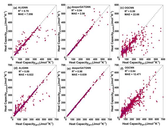
Fig. 8 Testing (top panels) and training (bottom panels) results of heat capacity for the three predictive graph neural network (GNN) models for 942 and 3769 structures, respectively: (a) ALIGNN, (b) deeperGATGNN, (c) OGCNN, (d) ALIGNN, (e) deeperGATGNN, and (f) OGCNN. The deeperGATGNN model shows the best performance for the testing (unseen) data.
