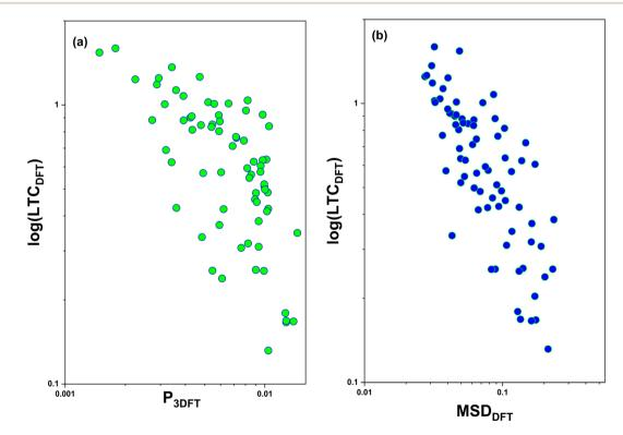
Fig. 6 DFT calculated LTC vs. (a)  $P_3$  parameter and (b) mean square displacement (MSD) for the 123 structures randomly chosen from the final dynamically stable structure pool (647) as screened by the workflow in this work.
