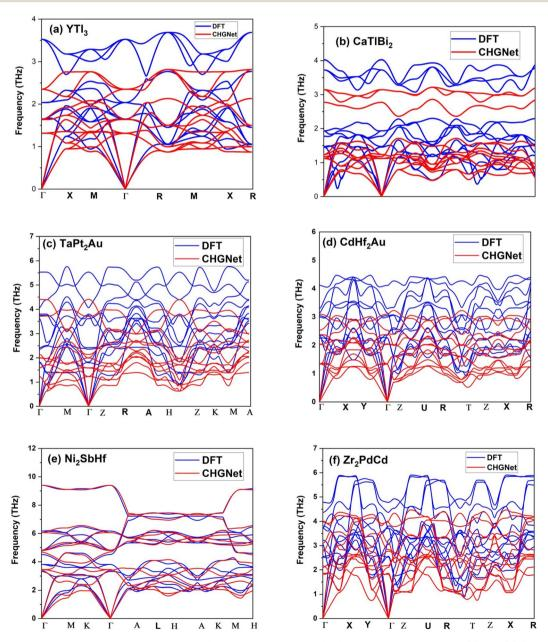
Fig. 3 Phonon dispersions along high symmetry paths of 6 selected structures by CHGNet and DFT calculations: (a)  $YTl_3$ , (b) Ca $TlBi_2$ , (c)  $TaPt_2Au$ , (d) CdH $f_2Au$ , (e)  $Ni_2Sb$  Hf and (f)  $Zr_2PdCd$ . The non-negative phonon frequencies by DFT prove the dynamic stability of the structures.
