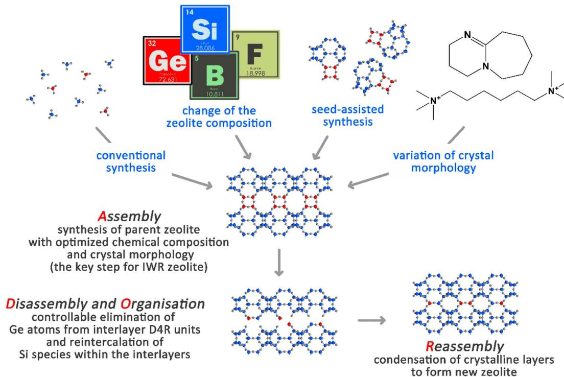
**Scheme 1** Schematic representation of the ADOR steps for the IWR zeolite under study. Ge atoms participating in the formation of D4R units in-between the crystalline silica layers are highlighted in red, while Si atoms are highlighted in blue.
