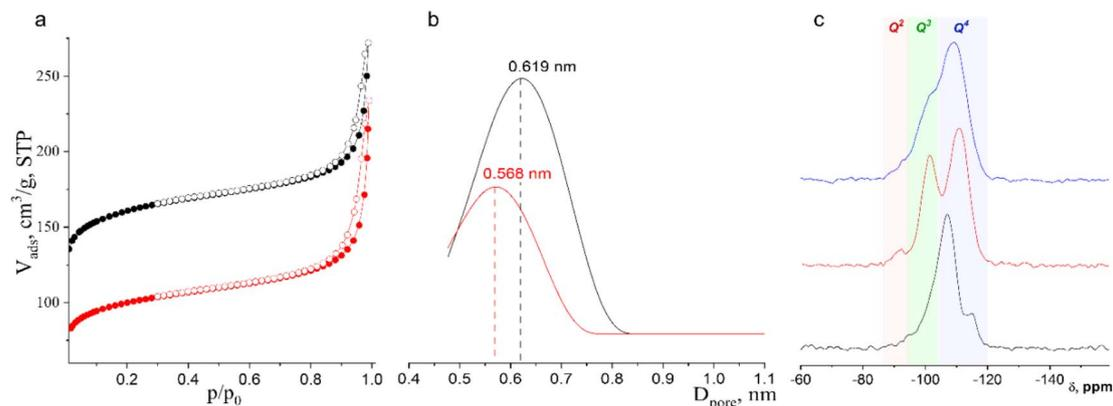
Fig. 4 (a) Argon adsorption/desorption isotherms for parent IWR and daughter IPC-17 zeolites; (b) pore size distribution of parent IWR (black) and daughter IPC-17 zeolites (red); and (c)  $^{29}\text{Si}$  MAS NMR spectra of initial IWR (black), intermediate IPC-17P (red), and IPC-17 (blue) samples.
