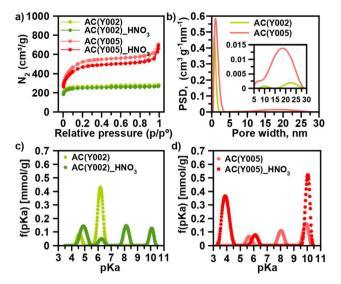
Fig. 1 Impact of HNO<sub>3</sub> oxidation on the pore surface of two representative microporous AC(Y002) and mesoporous AC(Y005) activated carbon spheres. (a) N<sub>2</sub> adsorption isotherms at 77 K. (b) Pore size distribution (inset: range extension between 5 and 30 nm). Distribution of acidity constants for (c) AC(Y002) and (d) AC(Y005) spheres before and after HNO<sub>2</sub> oxidation.
