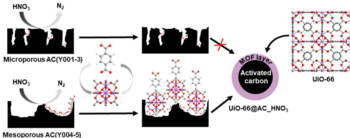
Scheme 1 Surface oxidation of microporous (top) and mesoporous (bottom) activated carbon spheres followed by layer-by-layer growth of UiO-66 thin films. Color code: oxygen, red; hydrogen, white; zirconium, purple; and carbon, grey.
