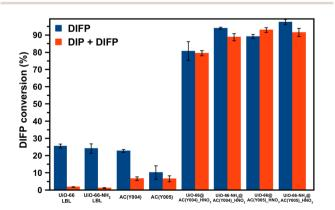
Fig. 4 Inhibitory effect of diisopropylphosphate (DIP) on diisopropylfluorophosphate (DIFP) hydrolytic degradation. Hydrolytic degradation of DIFP without the presence of DIP (blue) and in a 1:1 DIFP: DIP mixture (red) after 24 hours by the different materials.
