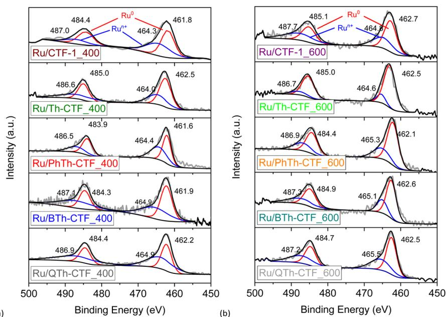
Fig. 6 High resolution X-ray photoelectron spectra of Ru 3p orbitals from (a) Ru/CTF<sub>400</sub> and (b) Ru/CTF<sub>600</sub>.
