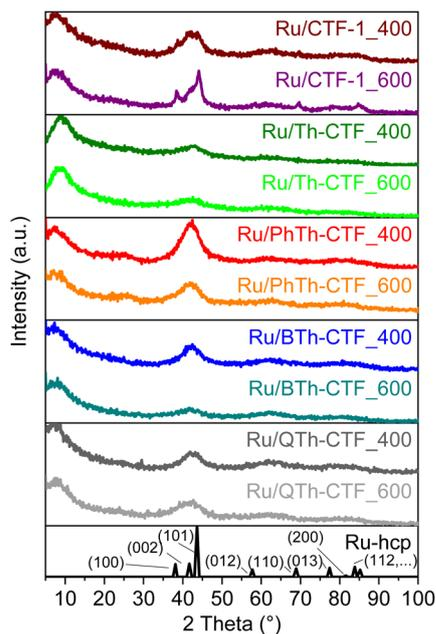
Fig. 2 PXRD patterns of the Ru/CTF composites. The simulated diffractogram of Ru-hcp with the assignment of the lattice planes corresponds to the COD 1512537 entry of the crystallographic open database.
