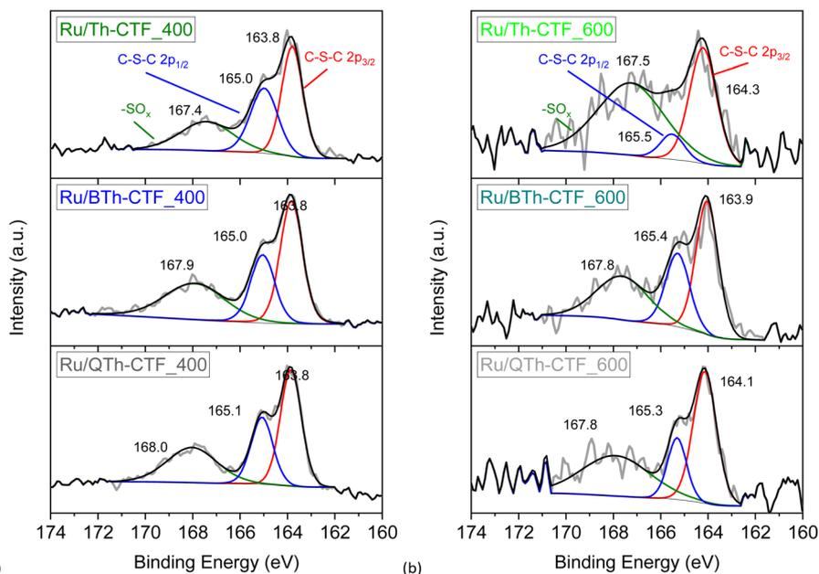
Fig. 7 High resolution X-ray photoelectron spectra of S 2p orbitals from (a) Ru/CTF\_400 and (b) Ru/CTF\_600. In case of Ru/PhTh-CTF the overall amount of sulfur (<1 wt%) is lower than the XPS detection limit.
